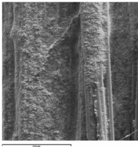
Micrography: Fibers inside the resin matrix arranged longitudinally
